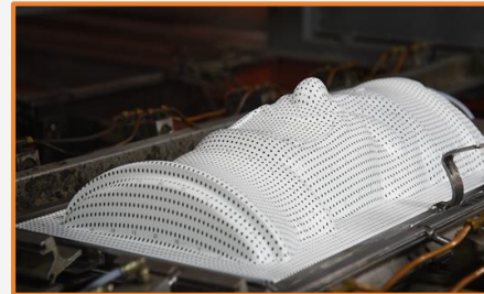
4. Some shapes require an image pre-deformation process to match the mold and artwork*.
